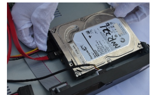
Figure3-2 Insert hard disk data cable and power cable
