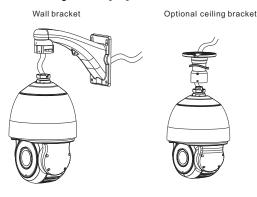
Step 3 Attach the high speed dome to the bracket, the tighten the three screws, as shown in figure 3-3.
