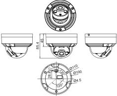
Figure 2-4 Dimensions of Large Dome(Unit:mm)
