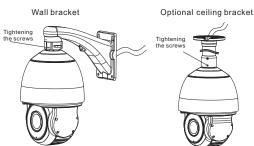
Step 4 Mount the high speed dome to the wall or ceiling and tighten the four screws on the bracket completely.
