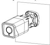
Step 4 Loosen the fixing screw and locking ring to adjust the position so that the camera faces the monitored area, then tighten the locking ring and the fixing screw, as shown in figure 3-2.
